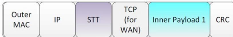
Figure 3 - STT encapsulation
